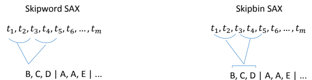
Fig. 4. Illustration of Skipword (left) and Skipbin (right) SAX. Skipword extracts the temporal correlation through using delay-time embedding vector in each single word; Skipbin captures the linear correlation in each word and preserves the sequential order in the PAA bins.
